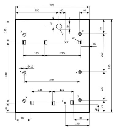
Prepare the tunnel for the power cable in the wall (corresponding to "Y" Hole in the slab).
