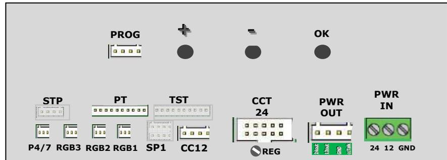
Get access to the menu by holding the three buttons pressed at the same time for 5 seconds.
