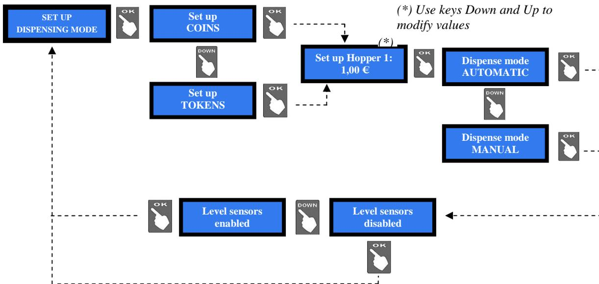
**NOTICE:** monitoring of level sensors is disabled by default. This means that the board does not know when the hopper is empty, so it will send the pay-out command even if there are no coins available. When the hopper runs out of coins during dispensing or at the end of payment, no warning will be displayed. If the empty state is detected when powering the unit, this one shall not accept any money.
