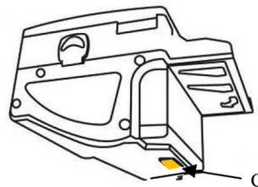
2. Move the D button upward, hold it while sliding the cover backwards; then lift the latter up and rotate it 180° to the right side.
