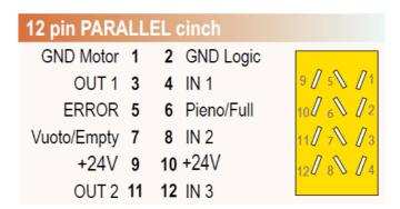
This connector can be found on the right side (**standard**) or left side (**reverse**) of the hopper. The functions of the pins will be described in the next paragraphs.
