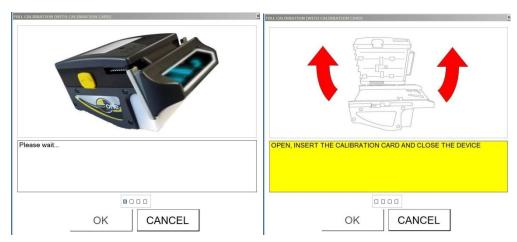
Once positioned the Calibration Card, press OK button and wait until confirmation of process ended.
